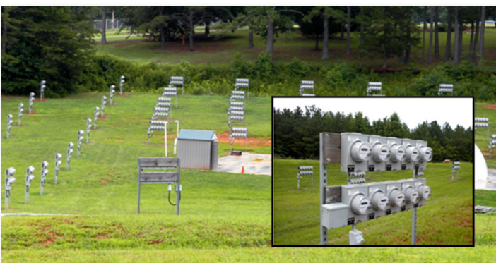
Figure 1 – Meter farm at the manufacturer’s facility with a rack of 10 smart meters in the inset.
