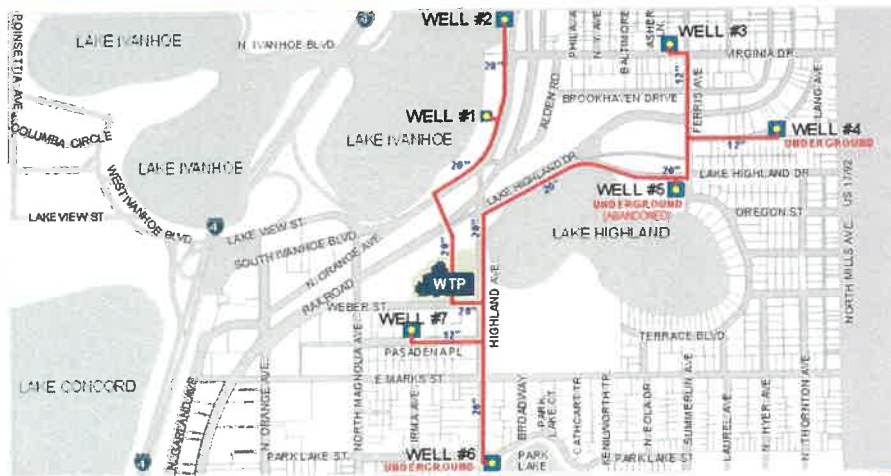
Approximately 4,100 feet of raw water piping will be replaced.
