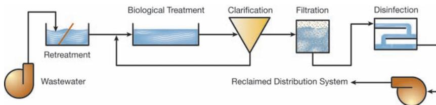
**How is reclaimed water produced?** Wastewater first undergoes pretreatment screening and grit removal, then undergoes biological treatment to remove organic material. The water is then clarified, filtered, disinfected and pumped into the reclaimed distribution system.
